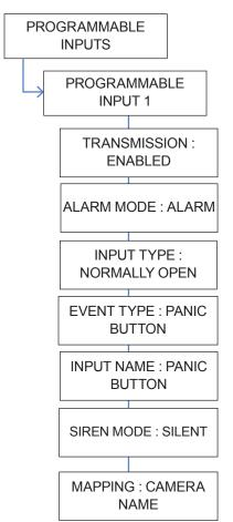
It is necessary to enable the transmission of the programmable input in order to transmit the event linked to the panic button.
