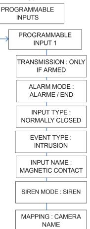
The main objective is to transmit events from the existing panel. It is important to select TRANSMISSION: ONLY IF ARMED in order to transmit only when the system is armed by the user.
