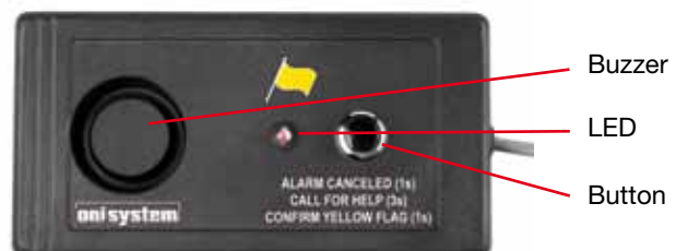
Dashboard panel (Yellow Flag, buzzer, button)
